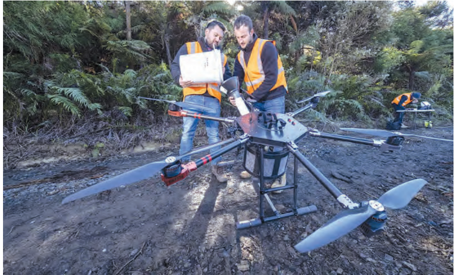
Envico founders Cam and Samuel loading seed pods into one of their heavy-lifting drones.
